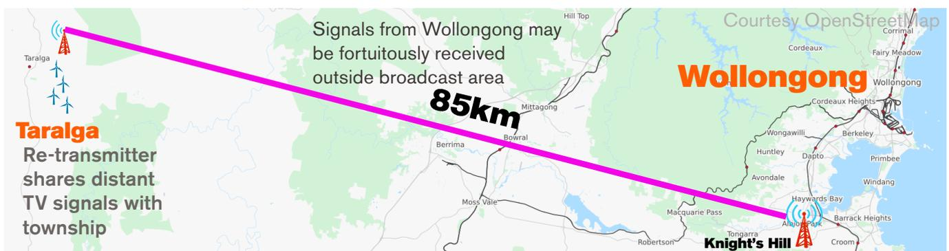
The Taralga wind farm re-transmitter receives a distant, fortuitous signal from Knight's Hill in the Illawarra area (85km away) for all free-to-air channels. The Taralga Wind Farm re-transmitter then re-broadcasts these channels to a small area, including most of Taralga township.
